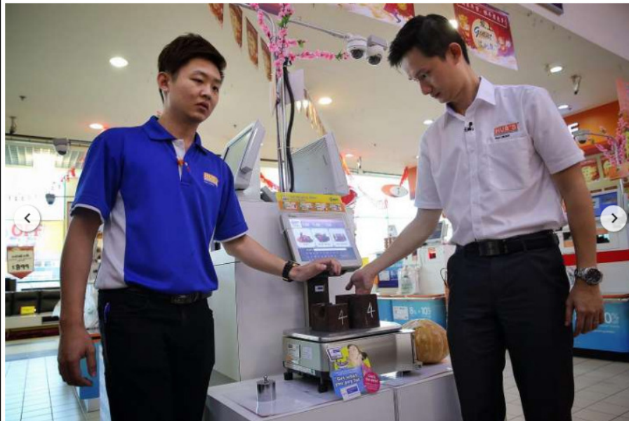
1 of 4 Spring-appointed authorised verifiers Mr Vincent Tan (right) and Mr James Lai (left) place calibrated weights onto a weighing scale as they demonstrate how they ensure the accuracy of weighing and measuring instruments. ST PHOTO: NEO XIAOBIN
