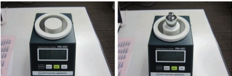
Annex figure 12: Check of the built-in scale
