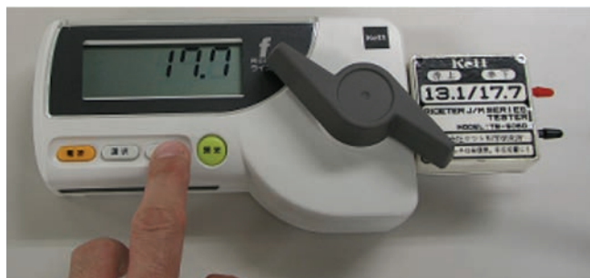
Annex figure 6: Check for the 17.7 % point by RfC
