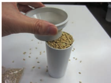
Annex figure 16: Pouring sample into a testing chamber
