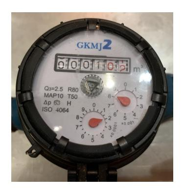
BRAND : GLMJ2 Q3 =  $2.5 \text{ m}^3/\text{ hr}$ Ratio = R80 DN15
