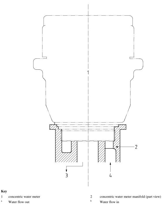
Figure E.1 Example of a manifold connection for a concentric water meter
