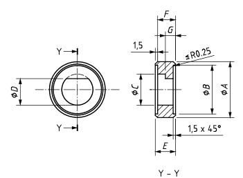
Machined surface roughness 3.2  $\mu m$  all over
