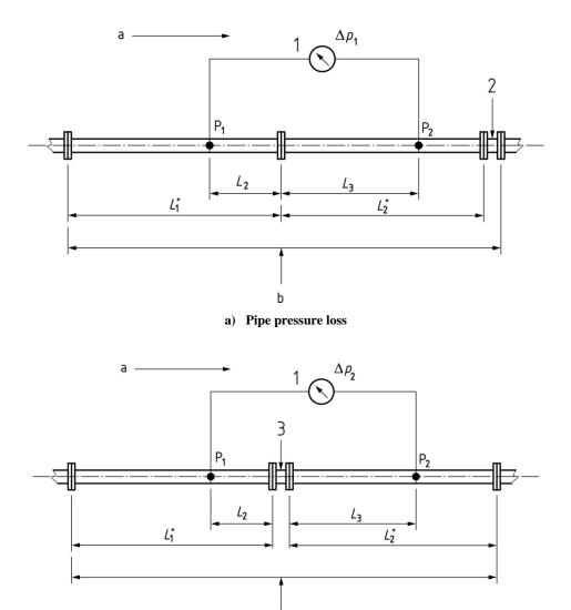
b) (Pipe and water meter) pressure loss
